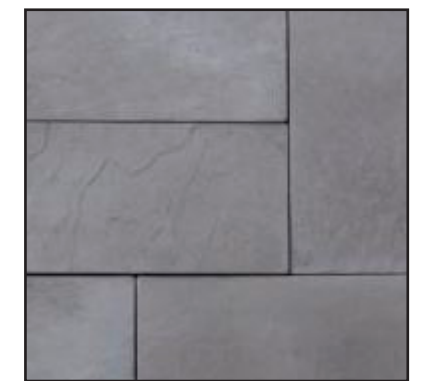
8. Bluestone Material: Bluestone to be installed at areaway in front of front door
